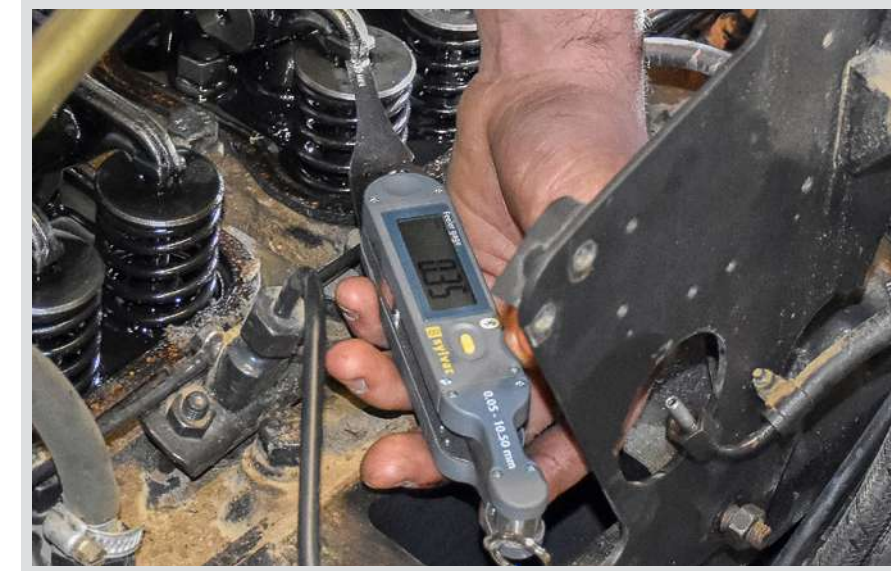
Measuring valves with Feeler Gage Smart
